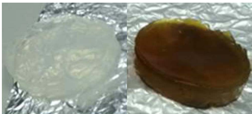
Figure 3. Neat PAM/PEI hydrogel (left); PAM/PEI-DSP hydrogel containing DSP (right). [Color figure can be viewed in the online issue, which is available at wileyonlinelibrary.com.]
